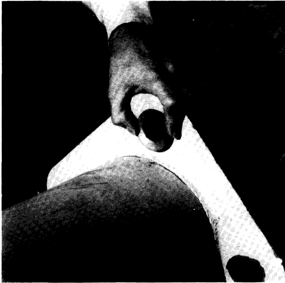
FIGURE 40 WASHER PARTIALLY EXTRUDED INTO HOLE
